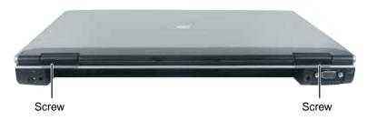
**9** Insert the small flat-blade screwdriver under the bottom of each hinge cover and gently pry it up.
